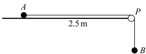
Two particles *A* and *B*, of masses 0.8 kg and 0.2 kg respectively, are connected by a light inextensible string. Particle *A* is placed on a horizontal surface. The string passes over a small smooth pulley *P* fixed at the edge of the surface, and *B* hangs freely. The horizontal section of the string, *AP*, is of length 2.5 m (see diagram). The particles are released from rest with both sections of the string taut.
